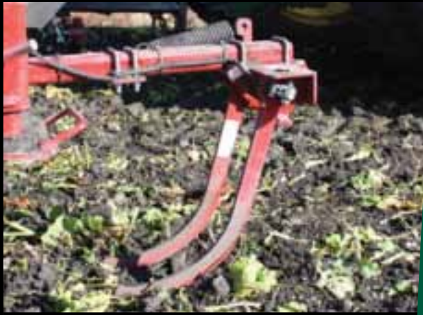
Active Depth Control wands continuously monitor ground conditions
