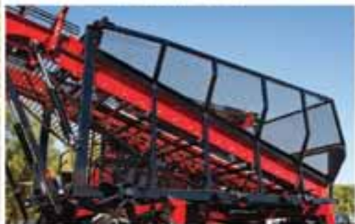
Large, 4.5-ton holding tank increases field efficiency
