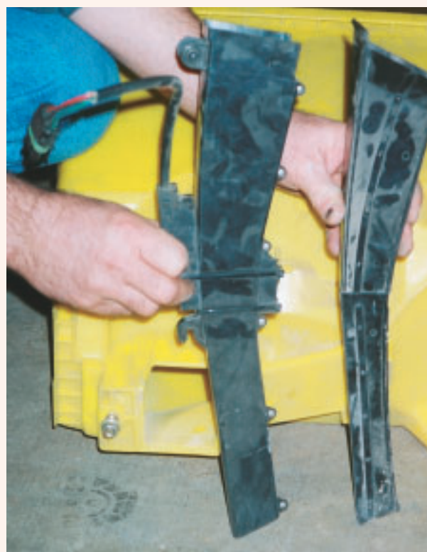
Above: Straight seed tube (left) and straight seed tube insert (right).
