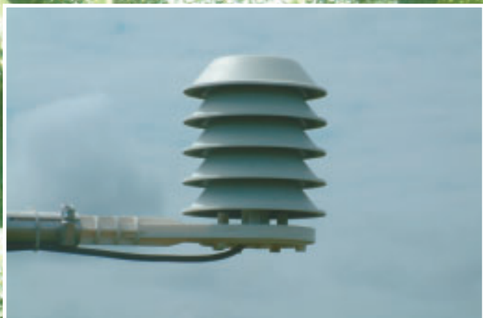
Left inset picture: The Ontario Weather Network's patented leaf wetness sensor used to determine hours of leaf wetness per day. Right inset picture: Commercial temperature sensor and housing used to capture temperature data.
