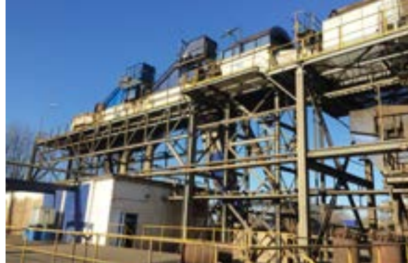
ABOVE The Rubanco factory's elevated beet washer, stone catcher and weed separator.
