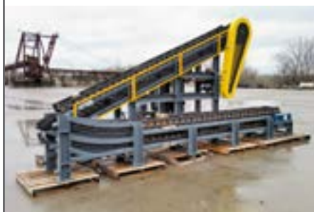
Pan conveyor (as delivered) replacing worn-out 1960s conveyors under the lime kilns.
