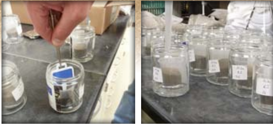
Figure 3. Measuring soil respiration in the laboratory to estimate nitrogen mineralization and microbial biomass.
