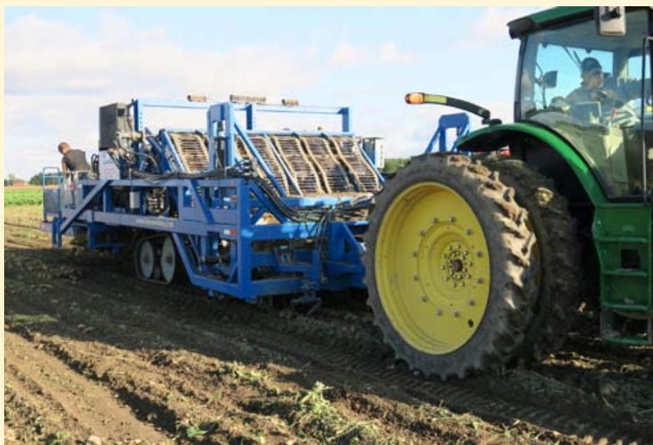
ABOVE: The research planter allows us to test a variety of seeds in specific settings, fungicides and other treatments we have available.
