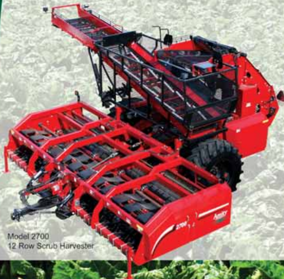
Model 2700 - 12 Row Wheel Harvester with industry-leading 42-inch-wide wheel.
