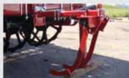
Wands mounted to the harvester send readings to the hydraulic system attached to the rear struts.
