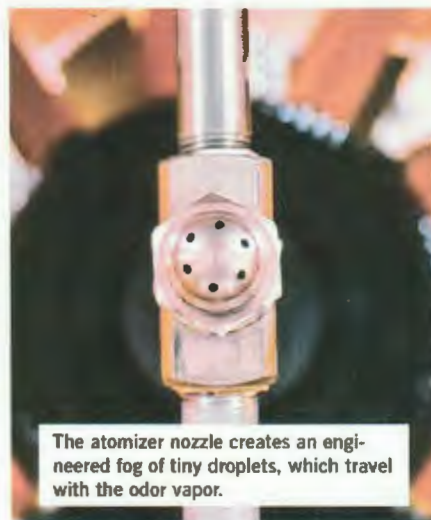
The odor control mixture is delivered through an open-ended barrel with a fan on one end and the Odor X Atomizer nozzle on the other.
