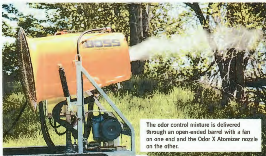
The atomizer nozzle creates an engineered fog of tiny droplets, which travel with the odor vapor.
